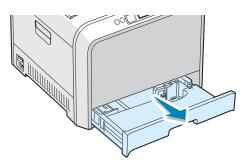
**2** Push down on the metal plate until it locks into position.
